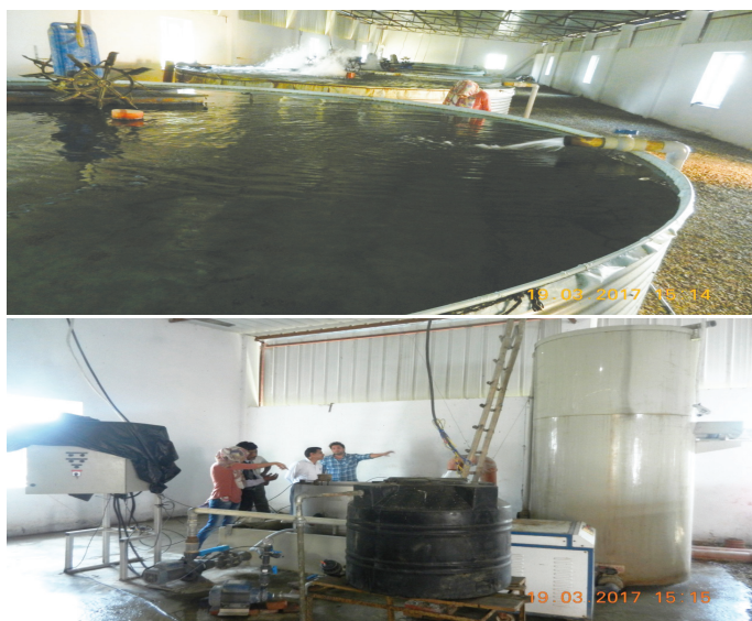
Indoor Recirculation Aquaculture System (RAS): Circular Tanks with aerators (above) and the Mechanical and Biological Filters (below), installed by Shri Neeraj Chaudhary at Sultan Fish Seed Farm, Butana village, Karnal district, Haryana State
